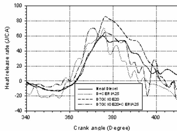
**Figure-5.** Variation of heat release rate with crank angle at the bmep of 0.44MPa.
