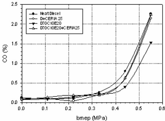
**Figure-6.** Variation of carbon monoxide with brake mean effective pressure.
