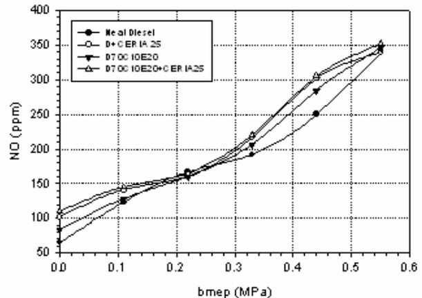
**Figure-8.** Variation of Nitrogen oxide with brake mean effective pressure.
