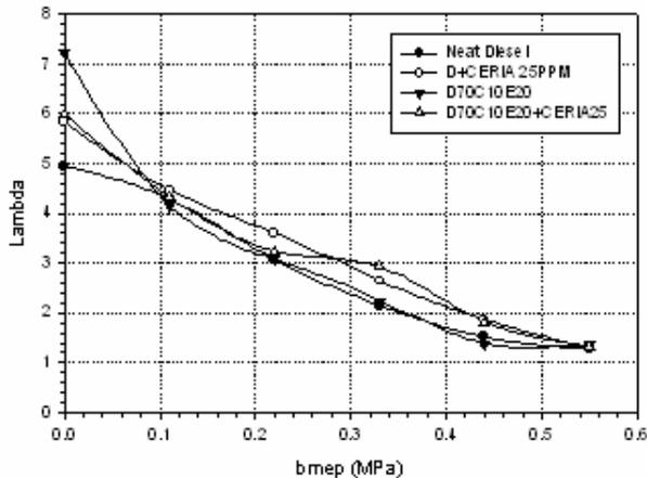
Figure-10. Variation of relative air fuel ratio with bmep.
