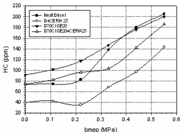
**Figure-7.** Variation of hydrocarbon with brake mean effective pressure.
