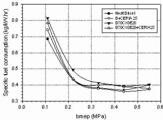
**Figure-2.** Variation of specific fuel consumption with brake mean effective pressure.
