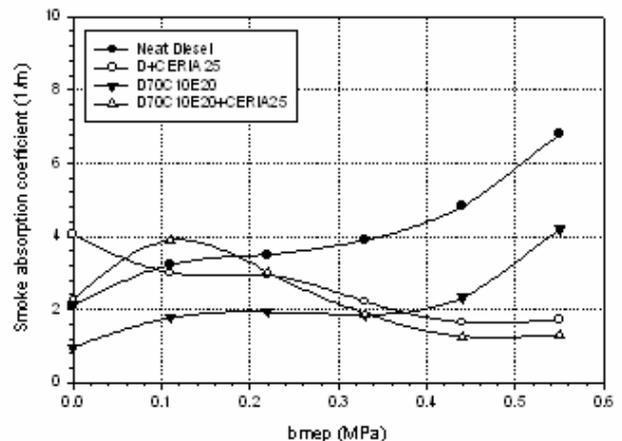
**Figure-9.** Variation of smoke absorption coefficient with bmep.
