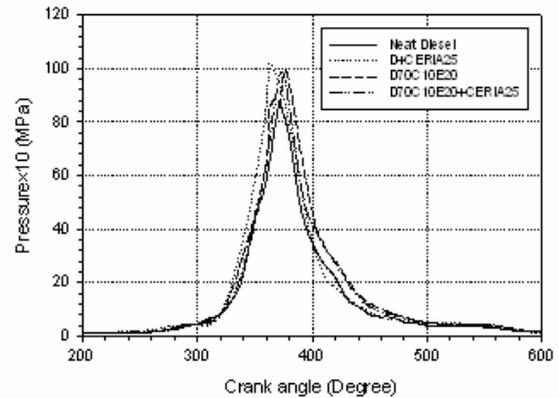
**Figure-4.** Variation of cylinder pressure with crank angle at the bmep of 0.44 MPa.
